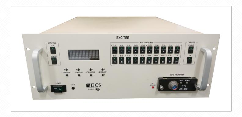
The Exciter incorporates state-of-the-art direct-synthesis technology to simultaneously generate up to 8 of 20 available standard IRIG tones. Complete configuration and real time control is provided via a front panel user interface, which incorporates discrete tone and carrier switches with indicators. Additionally the Exciter provides full remote control functionality via an opto-isolated serial port (RS422/RS232 selectable) or a discrete logic level interface port.
